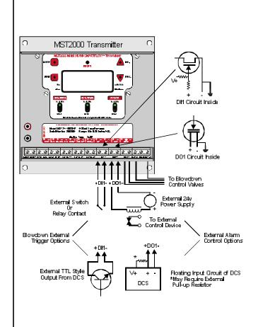
The DI1 (Digital In) connection accepts TTL level signals (isolated) or dry contact closures. If TTL signals are used, the ground connection <u>must</u> be floating and isolated from the 4-20mA loop connections.
